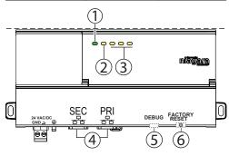
The controller has three yellow triac status LEDs, one yellow heartbeat LED, and a single green controller status LED located on the top of the controller. It also includes two LEDs for each Ethernet port which are located on the Ethernet connectors and are visible from the side of the controller.
