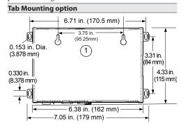
DIN rail mounting is recommended. Where tab mounting is required, use dimensions in the illustration to mount the controller.
