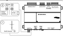
Because the Edge-10 uses a half-wave rectified power supply, it should not share a transformer with the JACE-8000, IO-R-34, or any legacy JACE.
