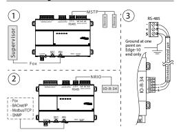
On the controller's top side, a single, non-isolated, RS485 port provides connection to IO-R-34 module or to other RS-485 devices (NRIO, MSTP, MODBUS). Do not use this port to connect to other JACE controllers.
