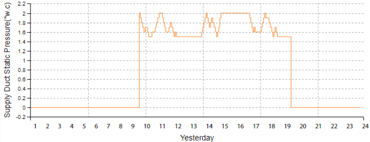
Static pressure SetPoint Reset
